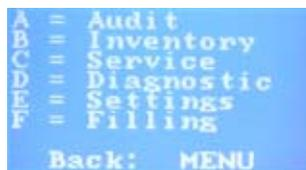
In the main menu for the coin changer currenza c<sup>2</sup> you select the submenu required by pressing the multifunction key with the character **A**, **B**, **C**, **D**, **E** or **F** on the left-hand side of the menu.
