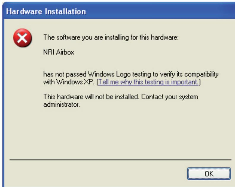
If you cannot complete the installation of the airbox driver, you have to change settings concerning the handling of unsigned driver software in the control panel:
