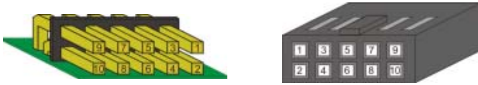
Figure 9: Lumina / SR5 ccTalk interface
